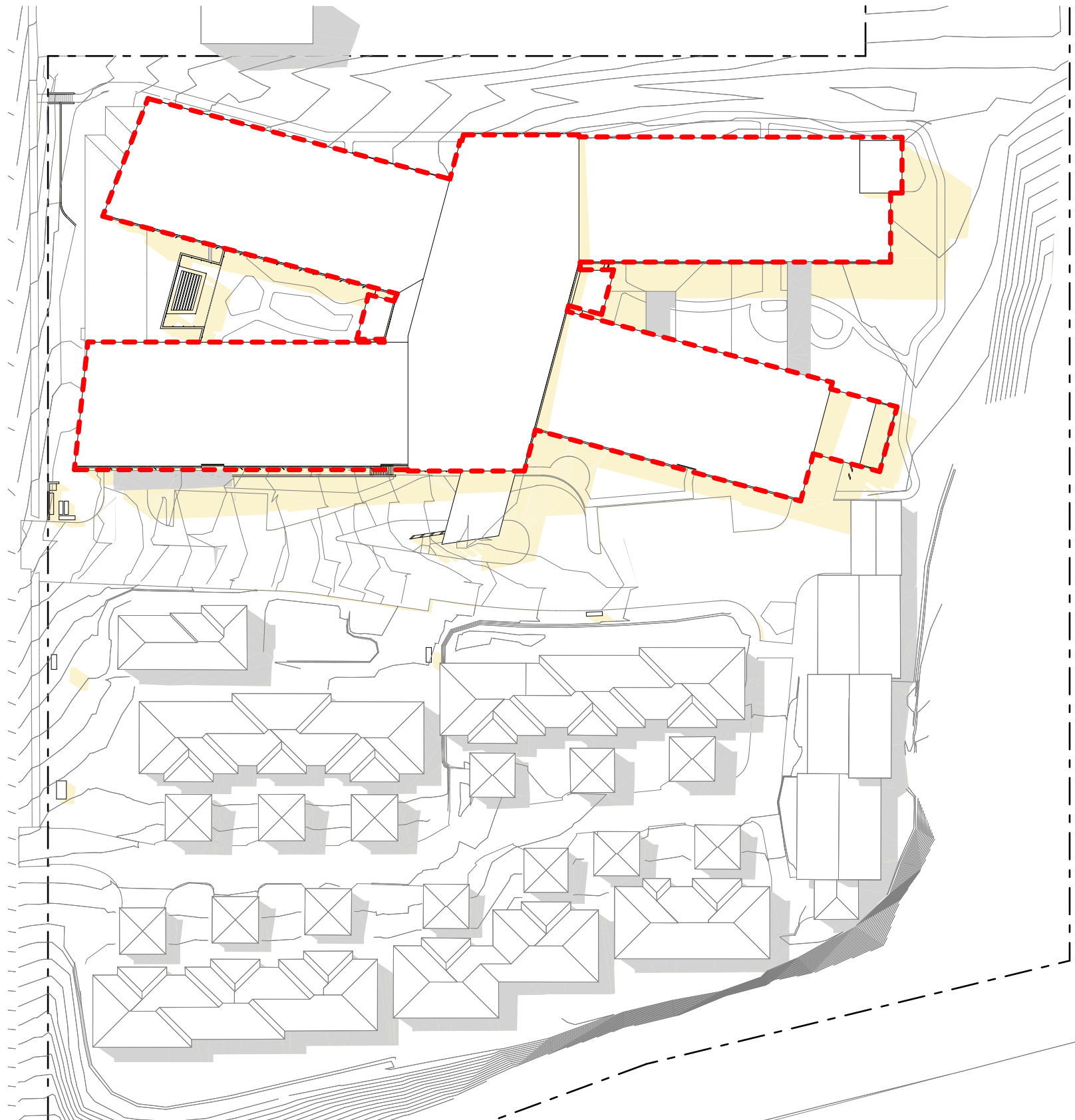
Shadow Diagram- June 21 12noon SCALE 1:750 @ A1
