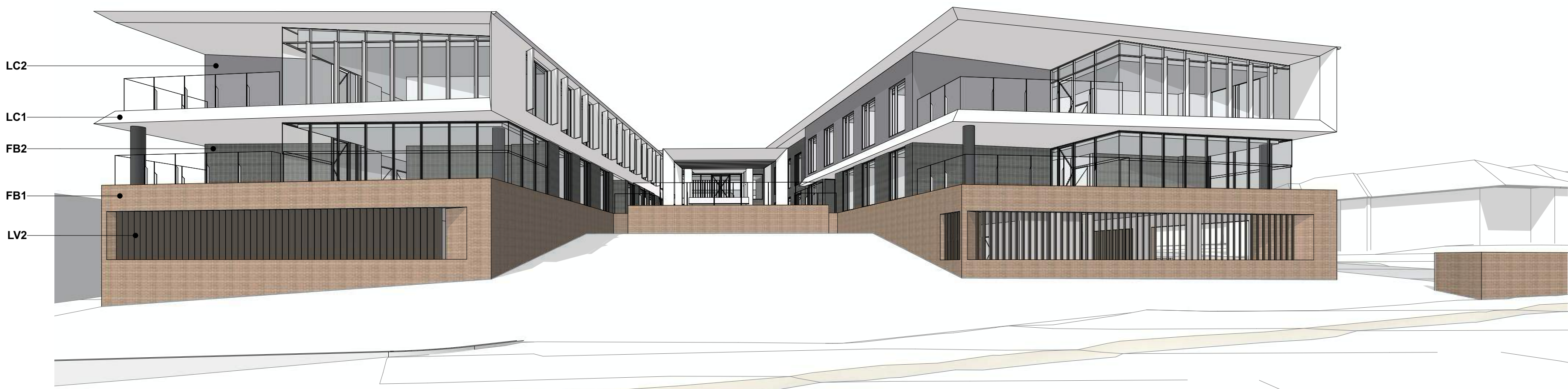
LC1 LIGHTWEIGHT CLADDING TYPE 1 LIGHT TONED VERTICAL CLADDING & SUNSHADES ALUMINIUM OR SIMILAR
