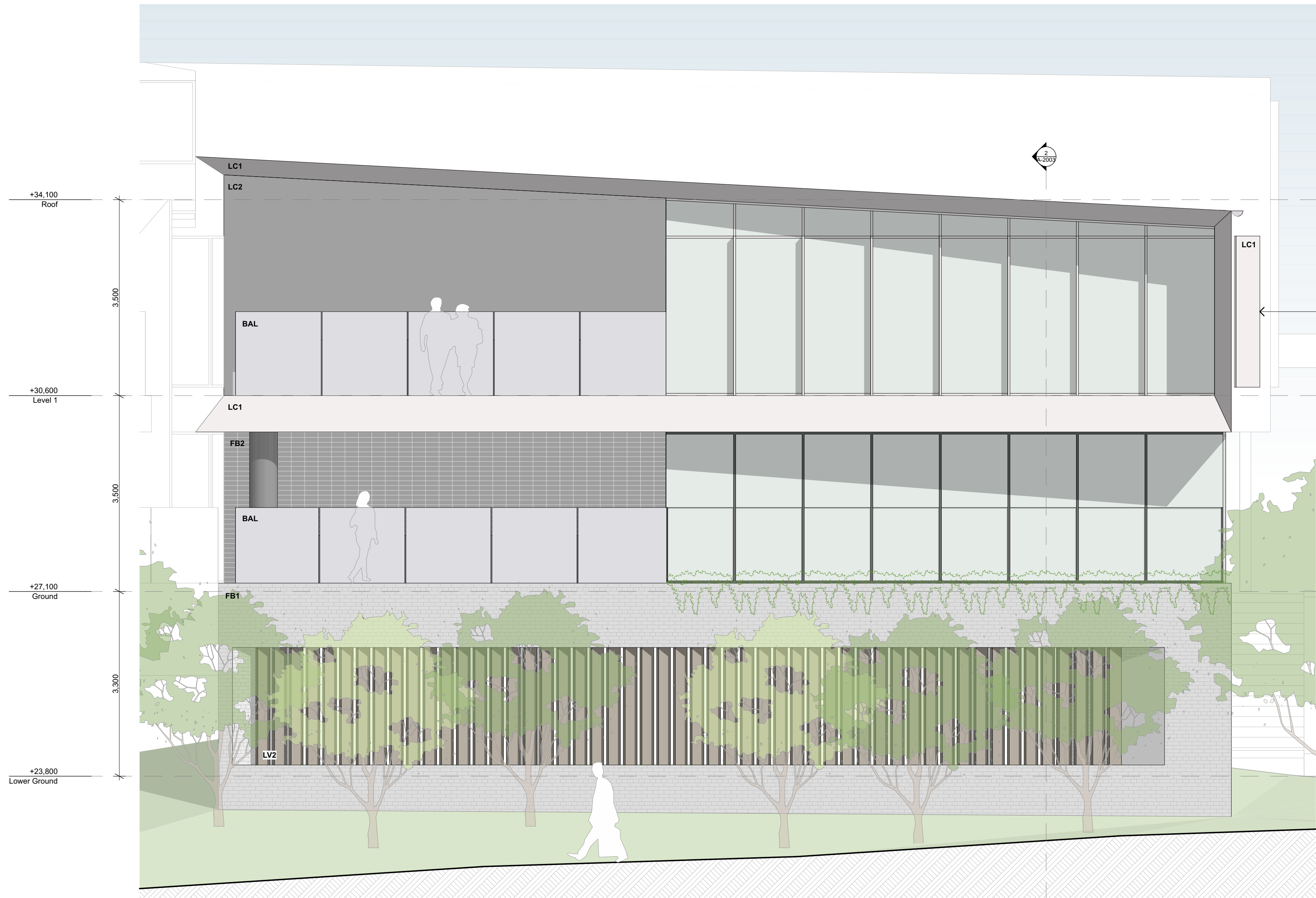
1 West Wing - True Elevation 1 SCALE 1:50 @ A1
